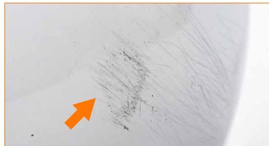
Visor with cuts and abrasions.
