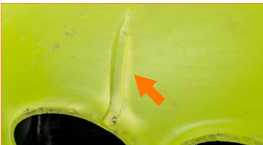
Shell shows impact damage in one place.
