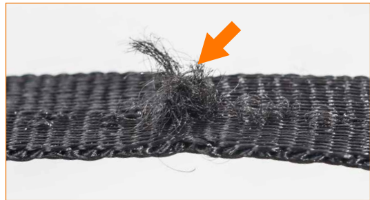
Threads unravelling from strap.
