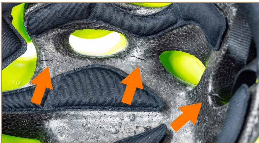
Internal polystyrene shell broken in several places.
