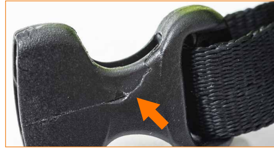
Female fastening clip broken.
