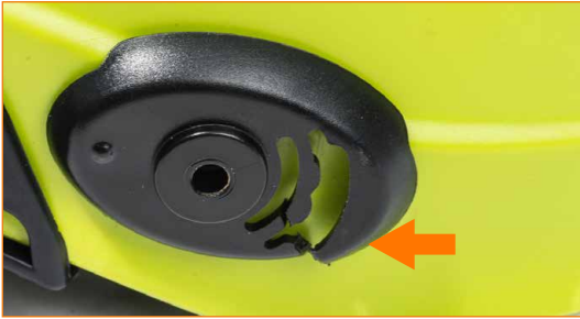
Visor support broken. 🔧 Replace with suitable spare part..
