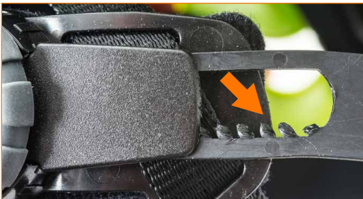
Headband adjustment mechanism has damaged teeth and doesn't stay in position.
